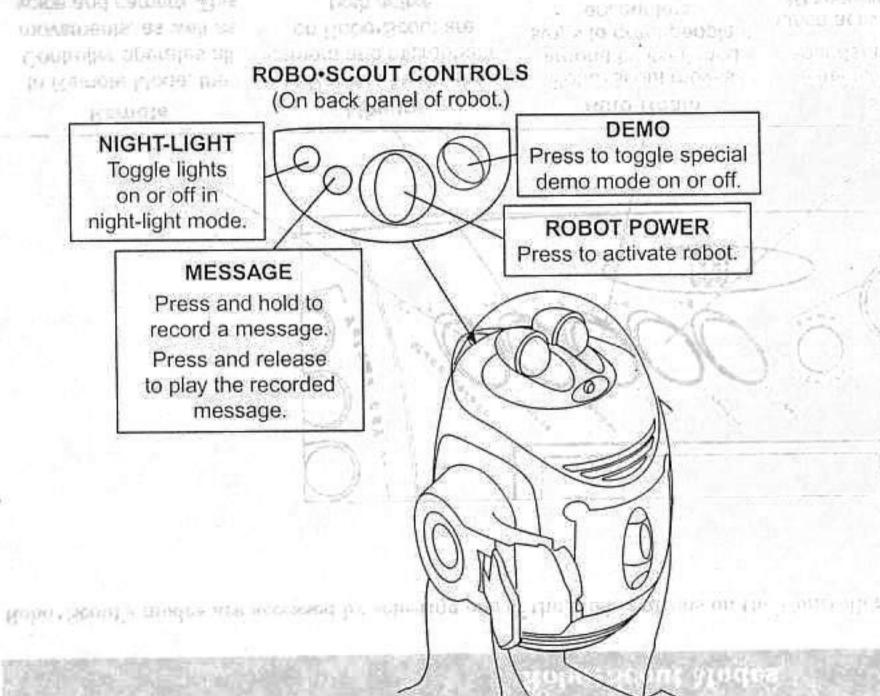
Robo · Scout and the Controller constantly communicate with each other whenever they are both powered up. If Robo · Scout is turned off, the Controller will shut itself off within two minutes to conserve batteries.
