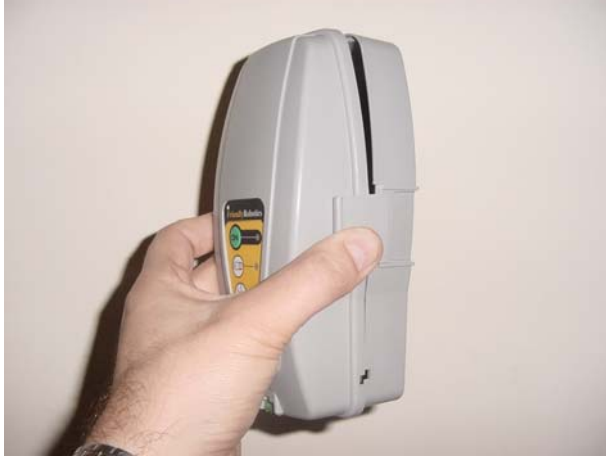
Figure 1.30 - Squeeze to remove cover
