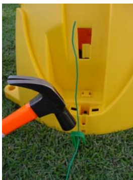
Figure 1.8 – Starting The Perimeter Wire in a Docking Station zone
