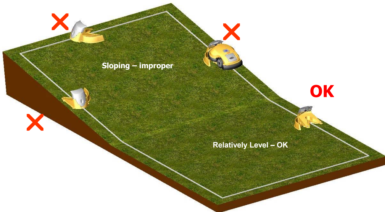
Figure 1.6 – Placing Docking Station on Level Ground
