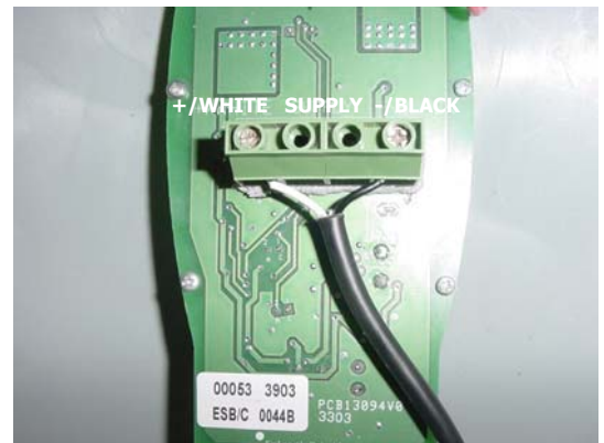
Figure 1.19 Power Supply Cord Track through the cover
