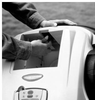
Figure 2.8 – Ground Clearance Location
