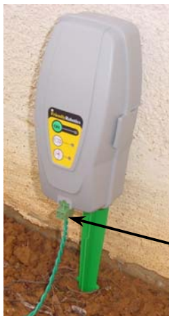
Figure 1.34 – Perimeter Switch with mounting stake attached
