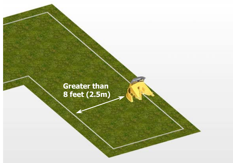
Figure 1.4 – Distance From Perimeter Wire
