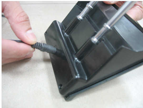
Figure 3.1 Power Supply connection to charging adaptor
