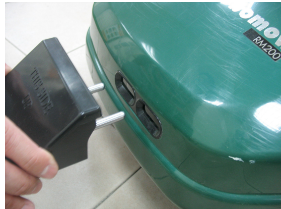
Figure 3.2 Charging adaptor connection to Robomow
