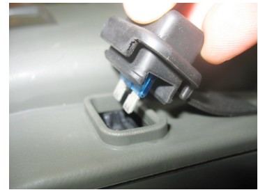
Figure 1.22 - Inserting batteries fuse
