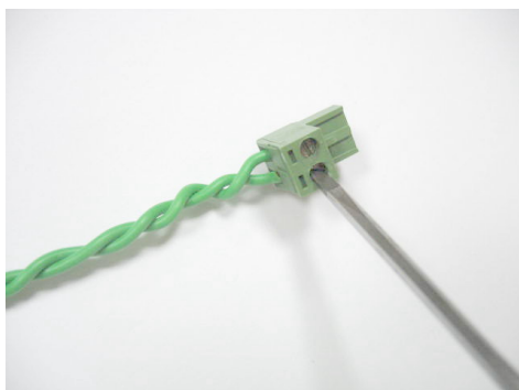
Figure 1.16 - Tighten the screw to secure the perimeter wire into the connector
